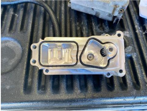
11.) Mount both halves together making sure to place the green gasket in between them in the proper orientation. Do not over tighten the retainers. Once they are tightened by hand evenly, it is now time to torque them. **TORQUE VALUE IS ONLY 25 IN-LBS.**
