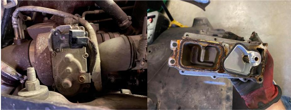
7.) Once actuator is removed, clean the surface of where the old actuator was mounted.
