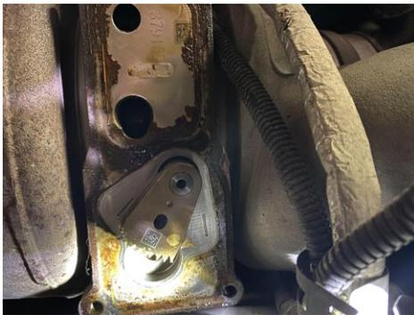
9.) Remove the 4 retainers that hold both actuator halves together. \*For 07.5-12 year models – you will need to separate the two halves and reuse the gear housing of the old actuator. Some of these may have tamper proof torx. For the 07.5-12 trucks, you need to make sure you get any water out of the gear housing before mounting the new actuator half to the old gear housing. If you get coolant in the actuator half for any reason you **WILL VOID** the warranty.
