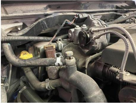
3.) Drain coolant. This can be reached from driver side after removing wheel & wheel liner. I found that by removing the driver side wheel & wheel liner it made it very easy to access the drain. You can also remove the lower radiator connection and drain it that way as well.
